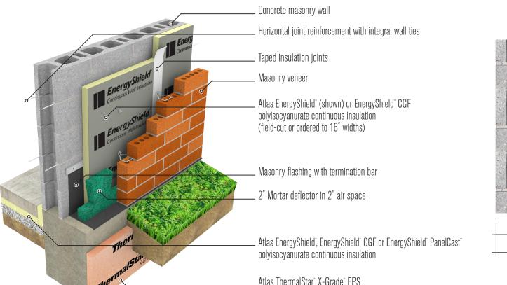
rigid continuous insulation at foundation
